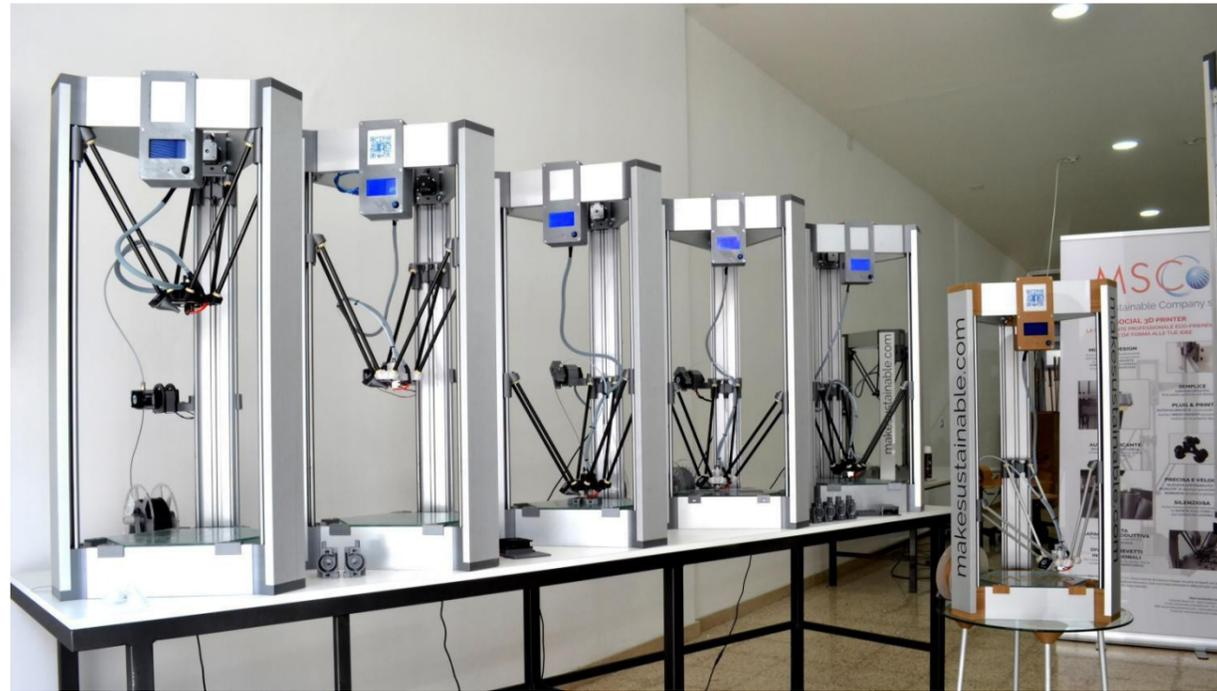
The **S3D PRINTERS** are **FDM** desktop printers (release of material on layers) with “**DELTA**” technology.
